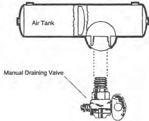
In addition to the three part air brake check, the following items must be inspected prior to operating a vehicle equipped with air brakes:
